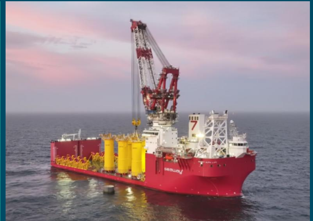
The Seaway Alfa Lift is a heavy lift vessel with a 51,000 dwt semi-submersible installation vessel of Ulstein design, which features a 3000t main crane and 10,000 m 2 free deck.
