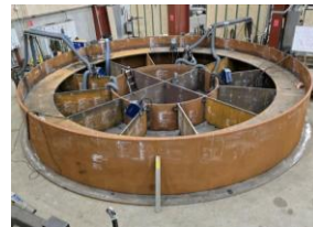
Centre column bottom plate
