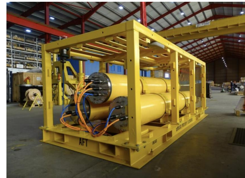
Example of subsea battery storage
